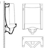
A fixing kit is supplied with the urinal. This comprises wall mounting brackets, water inlet connection for the flush unit and waste outlet connection to connect to the drain in the wall behind the urinal. Fixing Kit for UR1010 Code: UR1012
