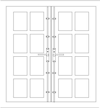
Joseph Giles Cremone Bolts are fitted with a unique non-handed rack & pinion gearbox mechanism which provides a 90 degree movement of the lever and a 13mm throw of the rods into the top and bottom of the door frame.
