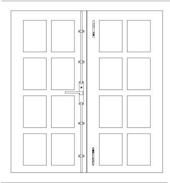
Joseph Giles Cremone Bolts are fitted with a unique non-handed rack & pinion gearbox mechanism which provides a 90 degree movement of the lever and a 13mm throw of the rods into the top and bottom of the door frame.
