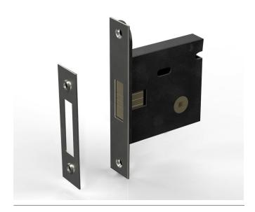
This sliding door look is recessed into the door and the dead-bolt is operated by a privacy thumb-turn from the inside and emergency release from the outside. When the thumb-turn is rotated, the bolt splays out sideways.
