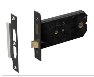
This horizontal privacy latch lock is recessed into the door. The latch-bolt is operated by a pair of door knobs and the deadbolt is operated by a privacy snib from the inside and emergency release from the outside.
