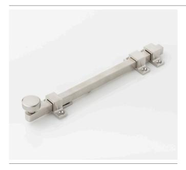
This solid brass surface-mounted skeleton bolt is usually fitted vertically onto the face of a door or window. It secures the slave door of a double door set to enable the main door to latch or lock into the slave door. Often used in conjunction with Cremone or Espagnolette bolts that have been fitted on to the main door.
