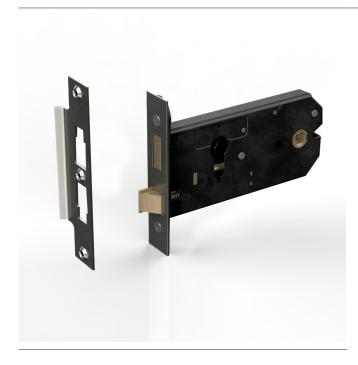
This horizontal latch lock is recessed into the door. The latch-bolt is operated by a pair of knobs or door levers and the dead-bolt by a key or thumb-turn in a Euro cylinder.
