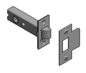
This tubular latch is recessed into the edge of the door and the latch-bolt is operated by a pair of knobs or lever handles. This latch is used for non-locking doors and ,may be paired with the LA1017 tubular bolt to create a bathroom door privacy set.
