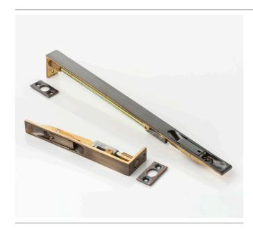
This lever action flush bolt is designed to be recessed vertically into the end or face of a door and is usually used to secure the slave door of a double door set; enabling the main door to latch or lock into the slave door. The bolt is thrown and retracted by operating the small lever.
