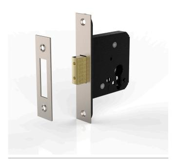
This deadlock is recessed in to the side of the door. Its dead-bolt is operated by a Euro cylinder with keys both sides or a key on one and a thumb-turn on the other. Euro cylinders are not supplied with Joseph Giles locks and need to be specified or procured separately.
